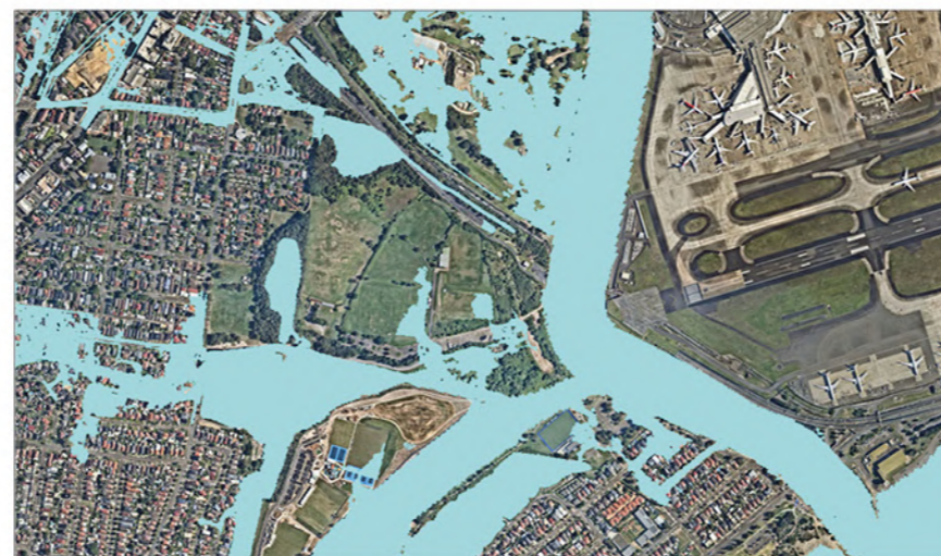
Figure 29 - 1% AEP Flood extent
